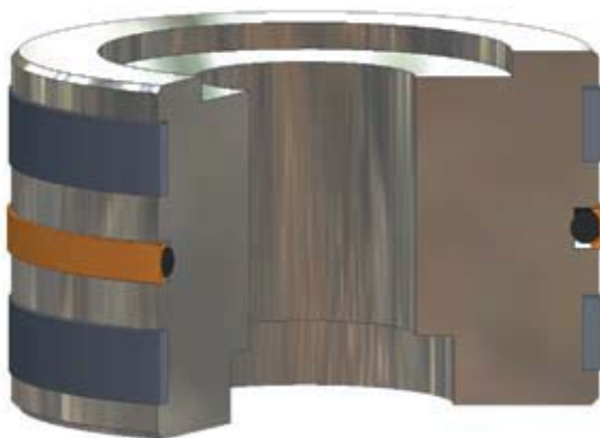
CP installed in Piston Gland
